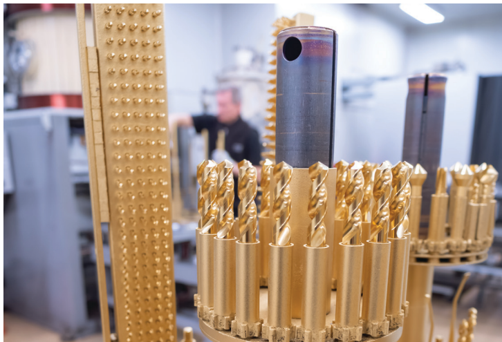
Drills receive Titanium Nitride coating
